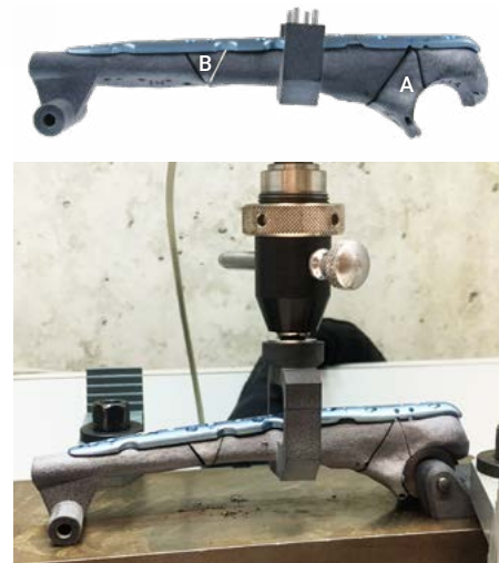
Figure 1: Test set-up (top: fracture lines, bottom: test set up on the machine)
