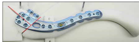
Fig. 2: Superior lateral plate setup, fracture line shown in red
